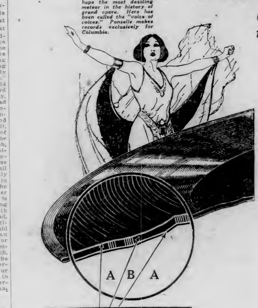
This illustrates the laminated construction of new process Columbia Records.
