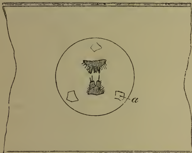
Fig. 127. Diagram illustrative of the method of mounting spinnerets, showing how they are to be arranged on the slide, and how the glass cover is to be prevented from unduly pressing them, by being supported on three bits of cover-glass ( a ).
