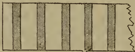
Fig. 141. Wood, with the strips glued on.
