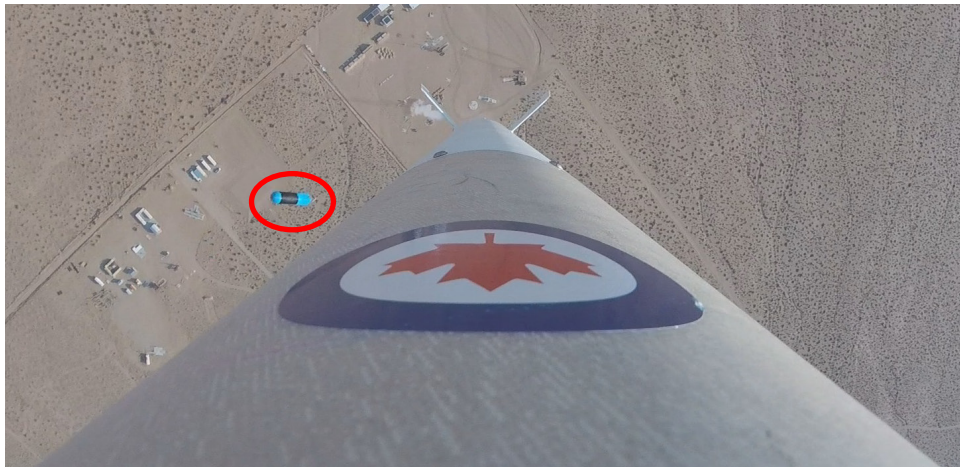
Figure 27. Front half of the bomblet falling away from rocket as seen by rear-facing camera mounted on rocket.
