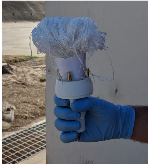
Figure 16. Initial kill mechanism design fitted with brass weights and packaged Dyneema net
