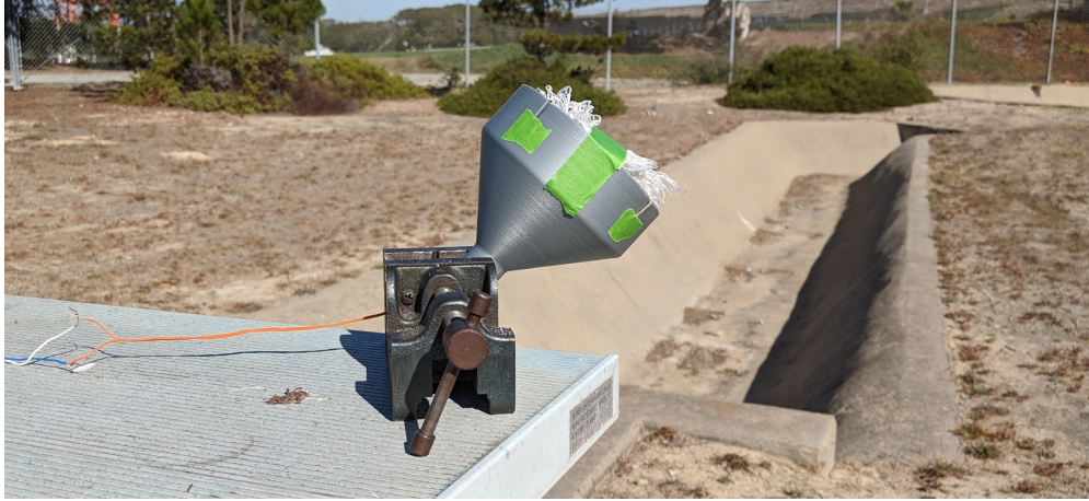
Figure 18. Second kill mechanism with net packaged in stowage space and held with tape.
