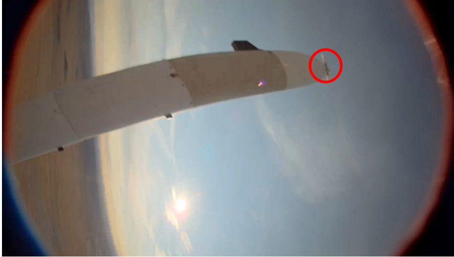
Figure 26. Servo section with partially deployed fins, remaining on the rocket, as seen from the submunition camera.
