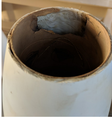
Figure 28. Gouging caused in the submunition stowage tube by the departing bomblet.
