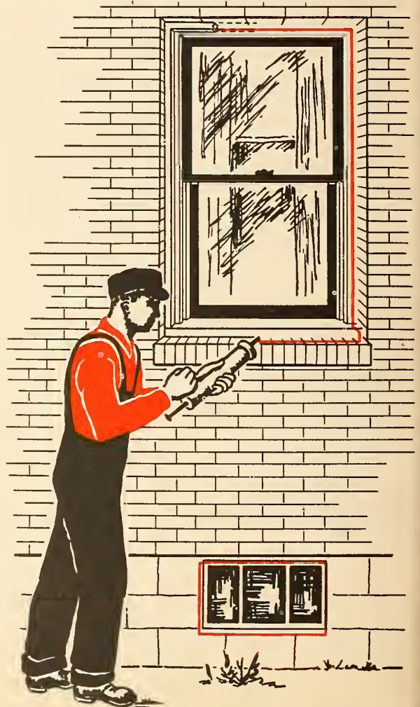
Figure 23.—Calking around windows closes air leaks.
