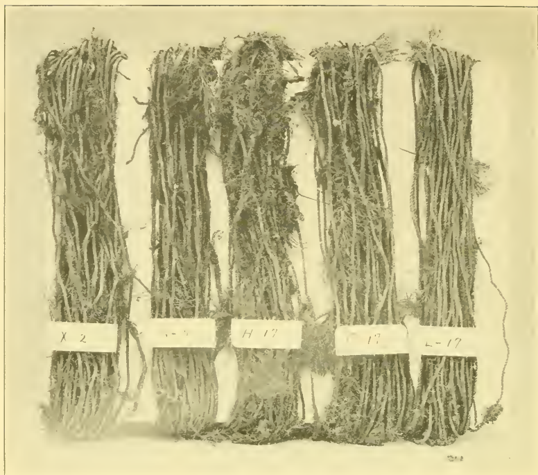
FIG. 18.—Cotton lines exposed in sea water at Beaufort, N. C. X, petroleum product No. 2, exposed one month; all the rest exposed four months. S, gilsonite; H, pine and coal tar; G, pine tar; L, Dutch method. All were somewhat fouled.
