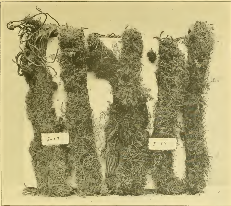
FIG. 16.—Cotton lines exposed in sea water at Beaufort, N. C., for four months. Heavily fouled. J, petroleum product No. 1; I, quercitron and potassium bichromate.
