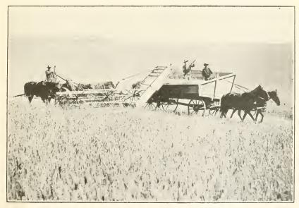
FIG. 2.—HORSE-DRAWN HEADER IN OPERATION.
