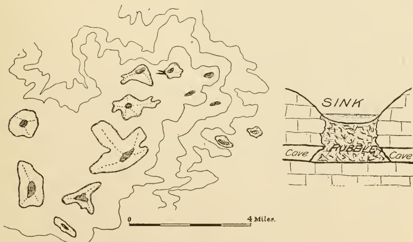
Fig. 9. Map and diagram to show manner of formation of lakes in sink-holes, (after Hobbs).
