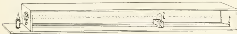
Fig. 2.—Apparatus for determining the principal focal distance through the observation of the conjugate focal distances. o , Object; i , image. The conjugate focal distances of o and i may be represented by f and f' respectively. c , Lens carrier which slides along the guide on the bottom of the box.
