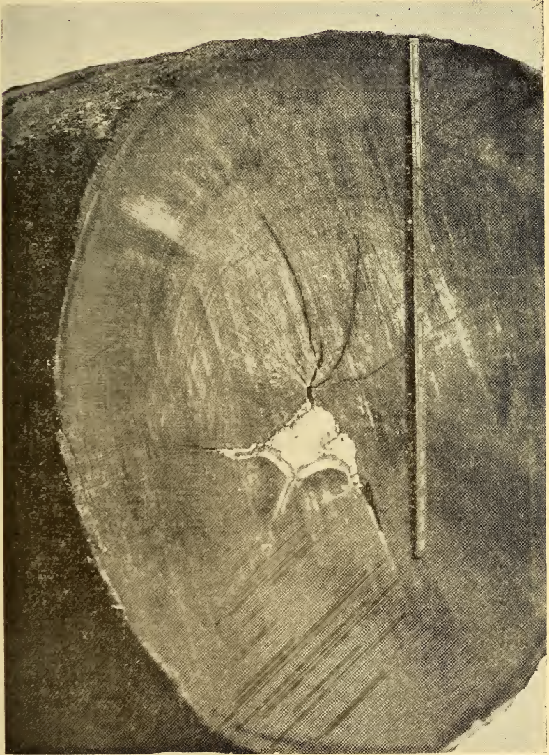
Log of Orites excelsa , showing deposit of aluminium succinate.
