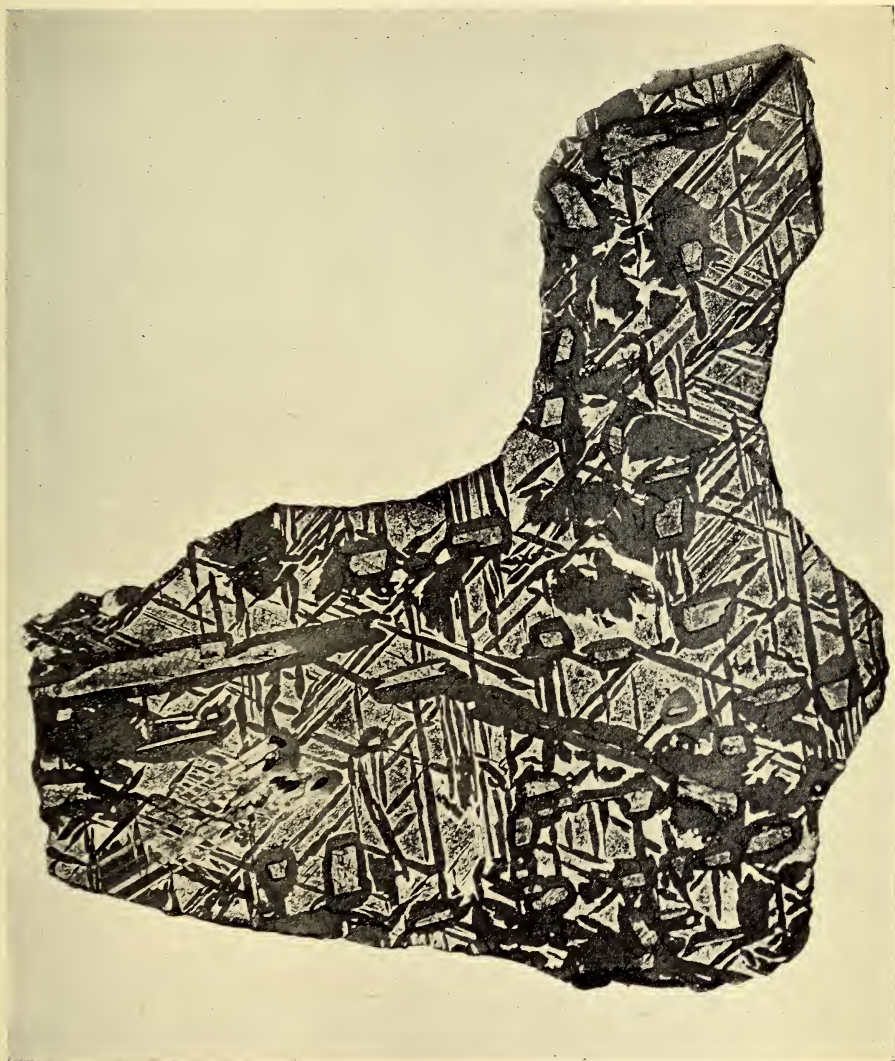
Section 1. Enlarged 2 dias. Etched by bromine water.
