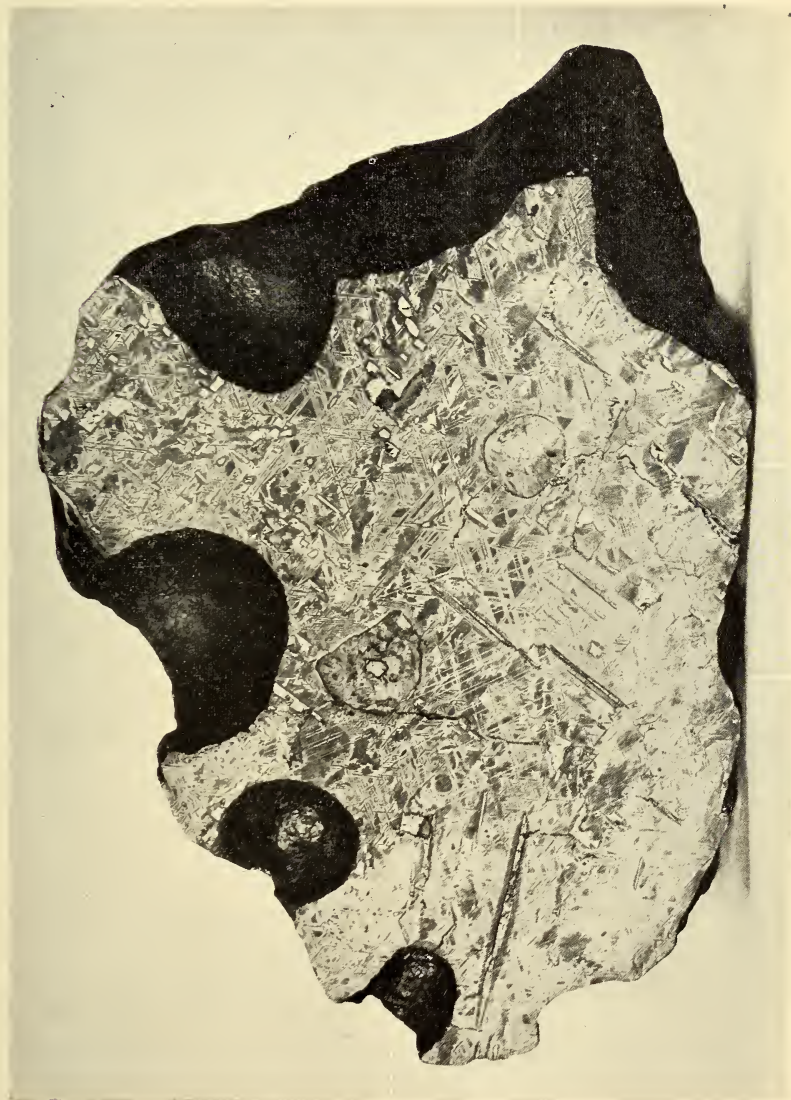
Section 8. \frac{1}{2} nat. size. Etched by bromine water.
