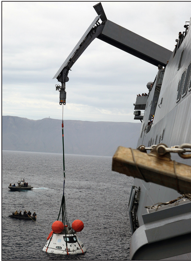
The Orion boilerplate test vehicle was lifted by crane from the water to test the proof-of-concept basket lift method Aug. 3 during a portion of Underway Recovery Test 2. Photo credit: NASA/Kim Shiflett
