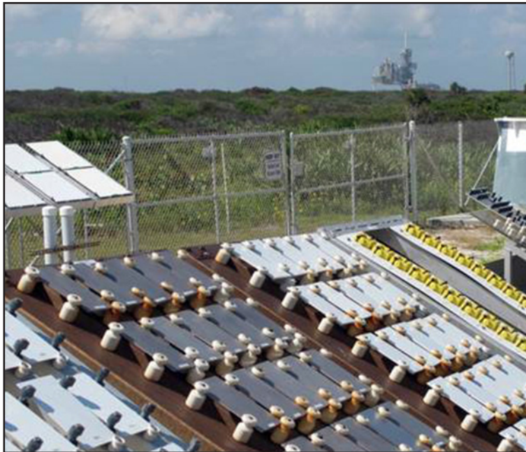
During Phase I testing, sets of stainless steel alloy samples were treated with citric acid and nitric acid and placed at the Beachside Atmospheric Test Facility at NASA's Kennedy Space Center in Florida. Photo credit: QinetiQ/Mark Kolody
