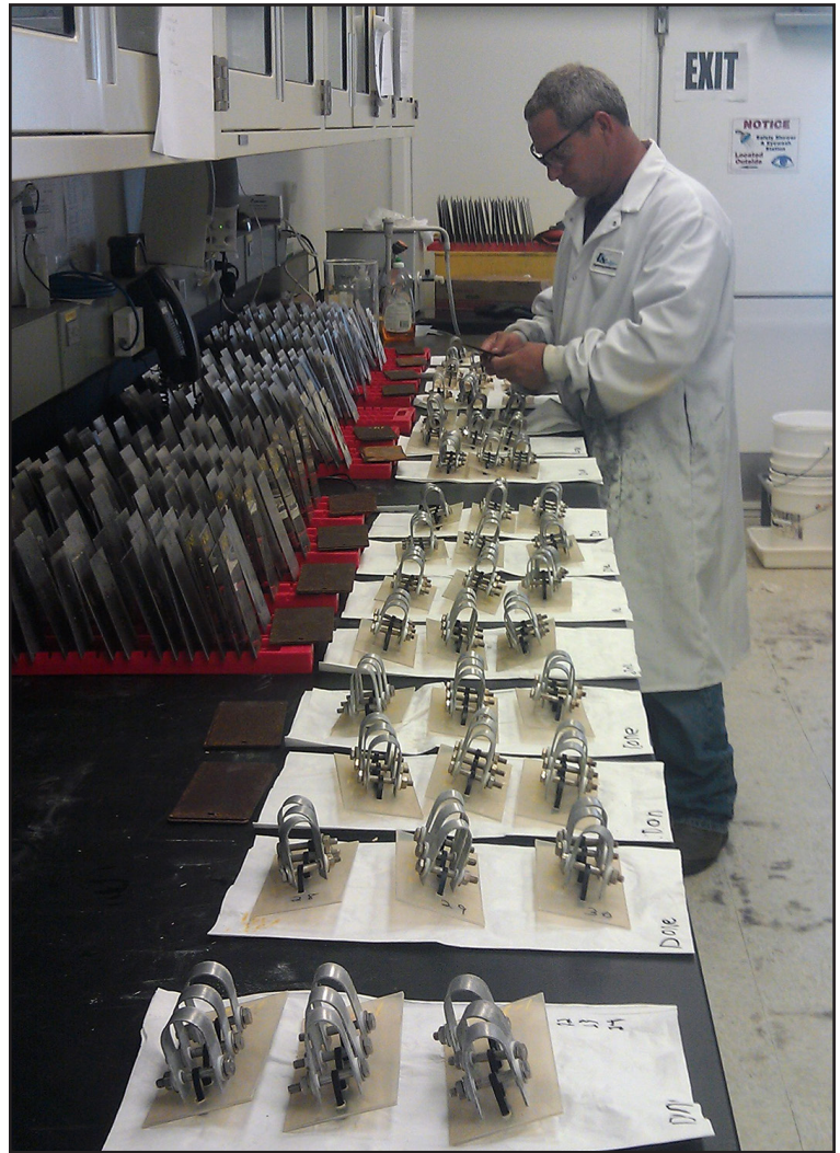
Teddy Beck, a corrosion technician with EASI, prepared bent samples of stainless steel in July 2013 for the stress corrosion cracking test in the Corrosion Technology Lab at the Operations and Checkout Building at NASA's Kennedy Space Center in Florida. Photo credit: QinetiQ/Mark Kolody
