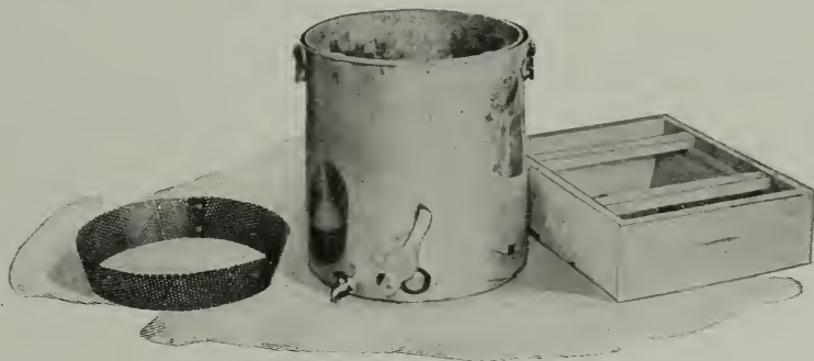
A simple form of capping-melter which consists of a can within a can, the space between being filled with hot water.
