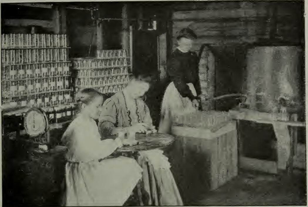
FIG. 3.—Filling and labeling bottles. The method of filling the bottles is here shown. The top label in the bunch is pasted, and the bottle rolled over it. Thus the labels are put on without being handled at all.
