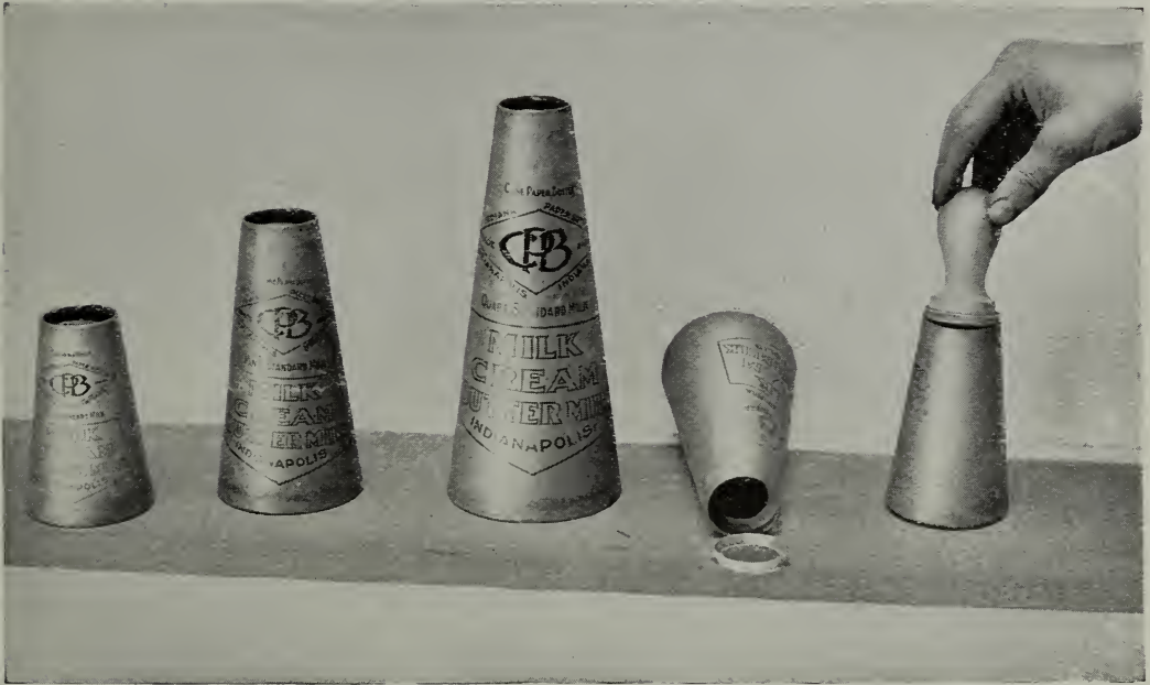
Fig. 3.—Samples of paper milk-bottles suggested by Walter S. Poucher, for retailing liquid honey. The stopper is crowded tightly into the small end with the wooden plunger. When clear in, it is impossible to remove the cap without the use of a knife or screwdriver. The cap is put on the small end to reduce the liability of leakage.
