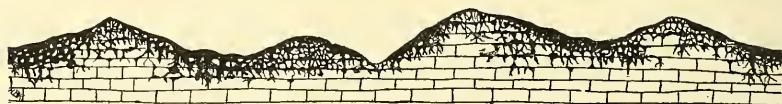
Fig. 4 shows relation of soil to rock, where the former has arisen by the decay of the latter. The line of contact is indefinite because of the irregular decay of the rock surface.
