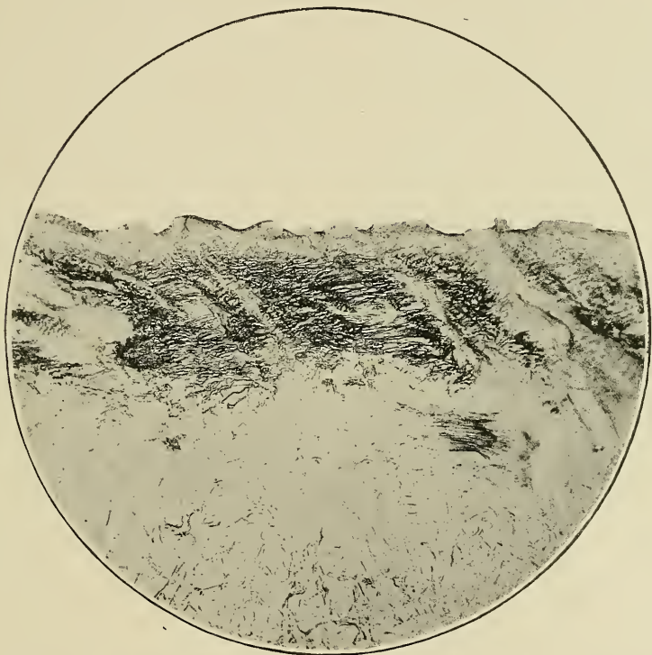
FIG. 41.—Butt of calf-skin after six hours' bating with trypsin. Stained as before.
