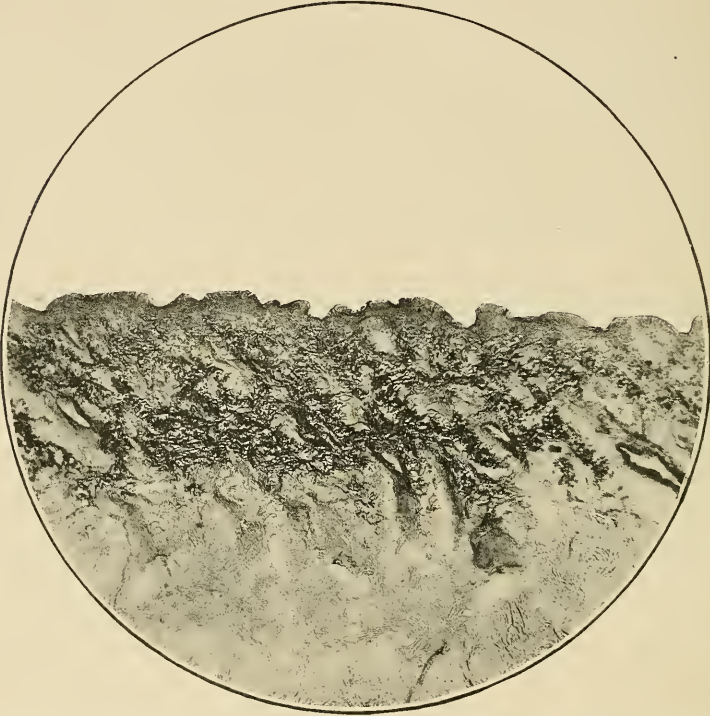
FIG. 40.—Butt of calfskin bated with ammonium chloride only. Elastin stained with Weigert's magenta.
