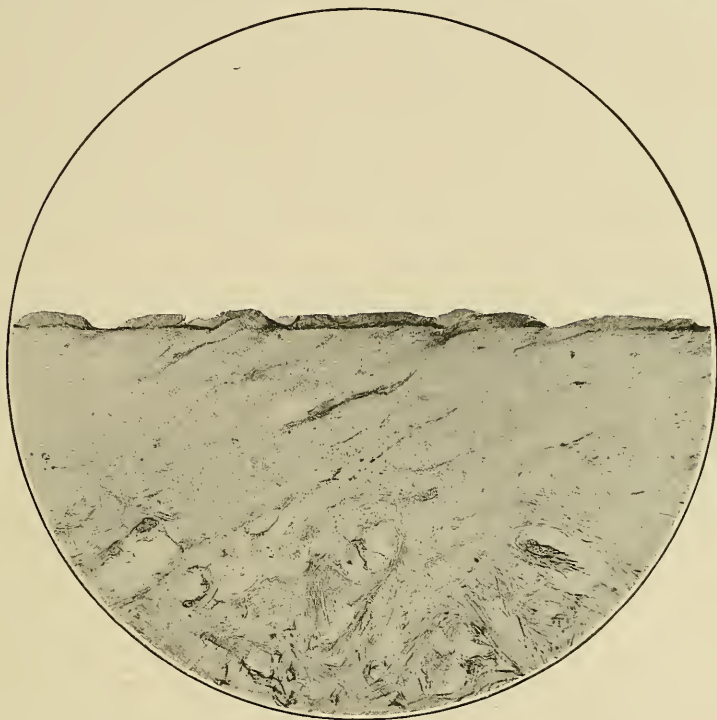
FIG. 43.—Butt of calf-skin after twenty-four hours' bating with trypsin. Stained as before.
