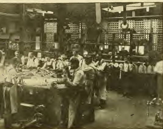
ASSEMBLING CONTROLLING STANDS
