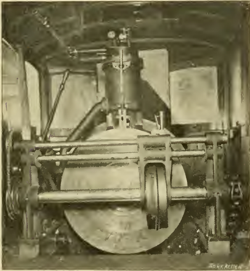
FRICTION DRIVE—CONNELLEY GAS MOTOR.
