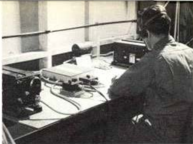
Controls of an interphone communication panel on a bomber installation.
