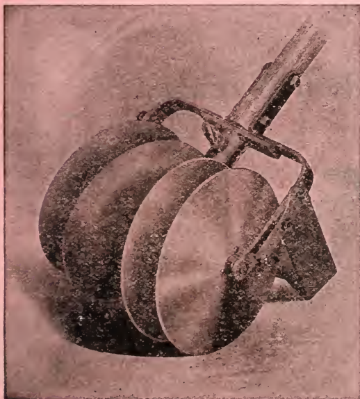
The Discs can be adjusted to an angle, throwing the soil to or from the plants
