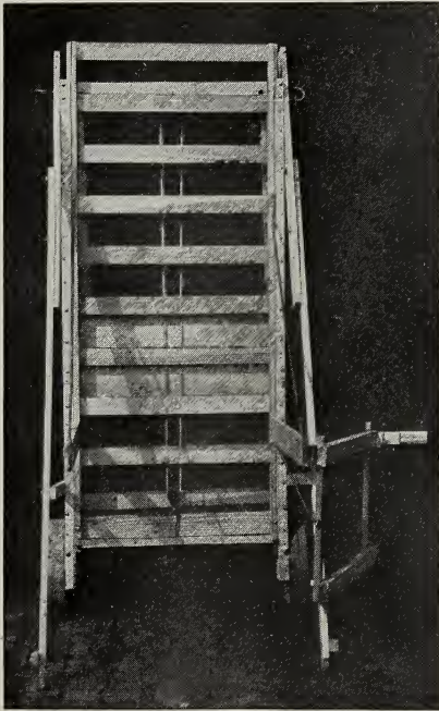
FIG. 13.—HIVE-HANDLING MACHINE; FRONT VIEW, AS READY TO BE SHOVED UP TO A HIVE.
