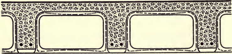
FIG. 43.—Pyrobar Gypsum Floor Tile.
