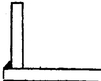
FIG. 17.—Single fillet used on a tee joint.
