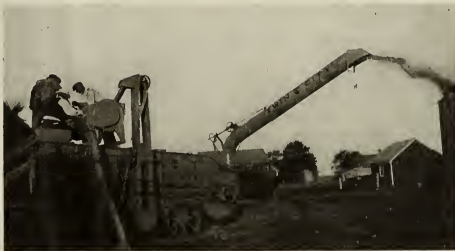
DISK GRAIN RECLEANER IN OPERATION ON THE DECK OF A THRESHING MACHINE
