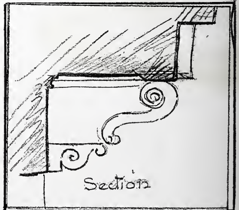
AN OLD CORNICE WITH DOUBLE BRACKET, SARAGOSSA.
