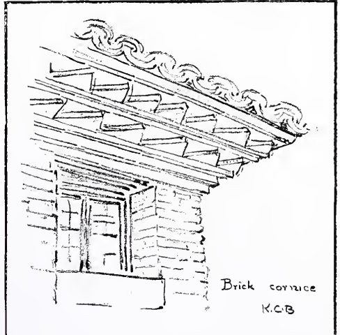
CORNICE OF UNUSUALLY LARGE BRICKS, WITH COURSES CORBELLED DIAGONALLY, FORMING A ZIG-ZAG PATTERN, SARAGOSSA.
