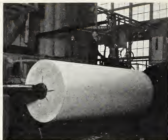
FIGURE 32.—Douglas-fir veneer log on lathe. The volume of Douglas-fir veneer produced in the region increased more than 250 percent during the decade 1927-36
