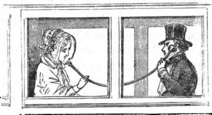
Fig. 60, Railway Conversation Tube.
