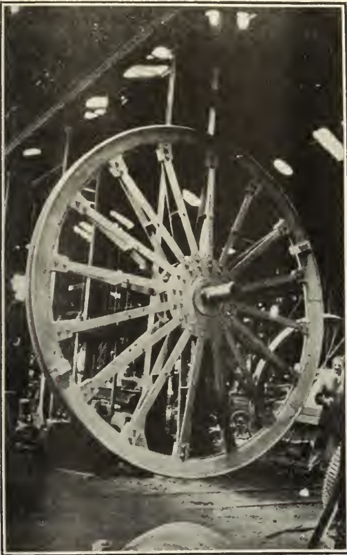
14 ft. Headgear Sheave for Brakpan Mines.
