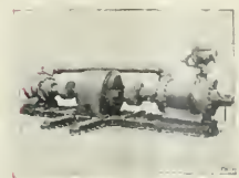
SULZER MINE PUMP.
