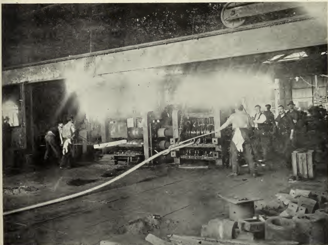
Rolling Reinforcing Rods 70 feet long in the 15 inch mill at the works of the Union Steel Corporation (of South Africa). Ltd., Vereeniging. The affairs of this highly progressive and successful enterprise, which has done so much for South Africa, are commented on in a leading article which appears in this issue.
