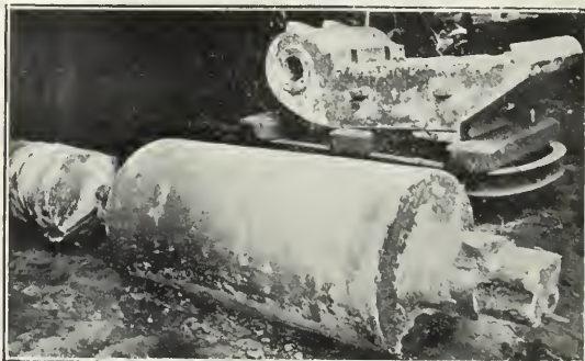
Pitman for Crusher, 2½ tons, and Roll for Steel Works, 2½ tons, cast by Rowe, Jewell & Co., Ltd.
