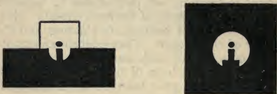
FIGURE 10. Correct Appearance of the Open and Peep Sights in Aiming.
