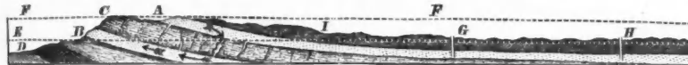
FIG. 8.—Section illustrating the failure of an artesian well because of defects in the confining bed below. A and B, porous beds; D and I, impervious beds; C, a defective confining bed; E, the water-level of the stratum B; G and H, wells that do not flow. The bed A might give a flow at G and H, but for the defect in C, which permits the water to descend into B and escape through its outcrop, which lies below the surface at G and H.
