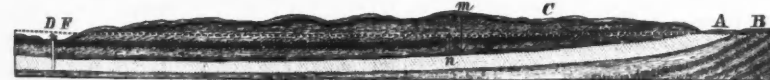
FIG. 9.—Section intended to illustrate the aid afforded by a high water surface between the fountain head and the well. A, a porous bed; B, confining bed below; C, confining bed above. The dark line immediately below the surface represents the underground water surface. Its pressure downwards is represented by the arrow m; the pressure upward due to the elevation of the fountain head is represented by the arrow n. The line F represents the level of the fountain head. There can be no leakage upward through the bed C except near the well D. There may be some penetration from C into A, which would aid the flow.
