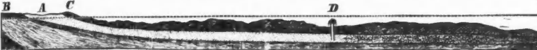
FIG. 5.—Section illustrating the transition of a porous water-bearing bed A into a close-textured, impervious one.
