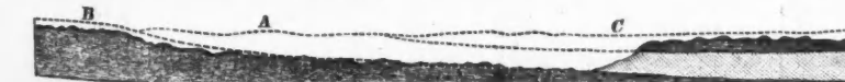
FIG. 13.—Illustrating a common effect of erosion upon the surface area of the porous stratum, and the contour of the resulting basin. Dotted lines show the original contours.
