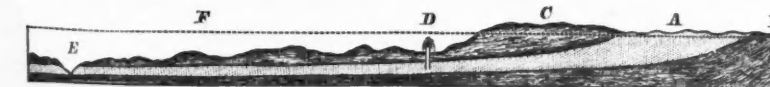
FIG. 11.—Section illustrating the possibility of a flow from a bed even when exposed at a lower level. A, a sandstone bed, thick and coarse at the right (its shore edge), and thinner and finer at the left; B and C, confining impervious beds; F, the water level in A; D, a well which may flow, notwithstanding the lower exposure at E.
