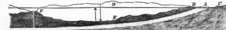
FIG. 10.—Double section illustrating the effects of high and low water surface in the cover area.
