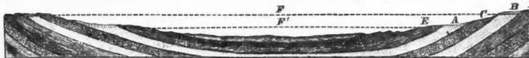
FIG. 6.—Section illustrating the usual order in which the strata of a basin come to the surface. A and B, porous beds; D and E, impervious beds; C, a half-impervious bed; F' and F, the water-levels of A and B respectively.
