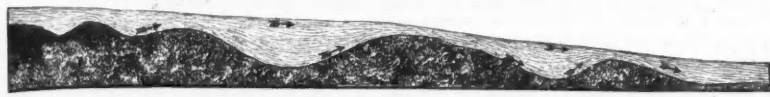
FIG. 1.—Longitudinal section of a stream illustrating in part its upward currents subordinate to the general downward flowing, and showing how water runs up hill.
