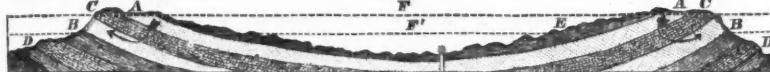
FIG. 7.—Section illustrating the possible effect of erosion upon strata originally like those in Fig. 6. If the stratum C is not practically a confining layer, the water from A will pass through it and escape at the edge of B, so that a flow can not be obtained at a higher level than it, but may be had below the line F'.
