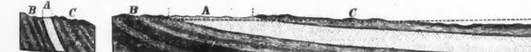
FIG. 12.—Section showing the difference between a highly inclined water-bed and a gently tilted one in catchment area at the outcrop.
