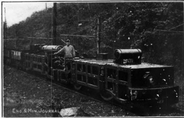
30-TON DOUBLE-UNIT ELECTRIC MINE LOCOMOTIVE
