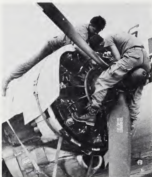
Department of Defense Photo (USMC) A421998 Cpl William H. Mielke (top) and LCpl Phillip J. Orlando of Headquarters and Maintenance Squadron 36 repair the AD20-8 engine of their squadron's C-117D at Phu Bai on 30 December.
