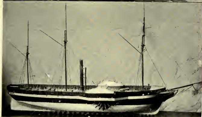
MODELS OF H.M. PADDLE SLOOP "RHADAMANTHUS," SHOWING (1) DECK DETAILS AND ARTISTIC FIGUREHEAD; (2) BROAD- SIDE OF VESSEL
