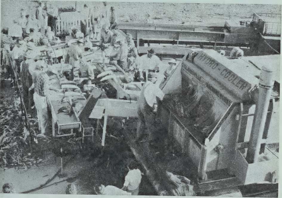
Hydro Cooler and Grader processing sweet corn at the Horticultural Station at Brooks.
