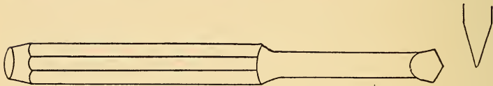
Fig. 63. The granite hand drill, illustrating flat and side views of the bit.
