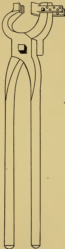
Fig. 4. Adjustable tongs regulated for holding largest size.
