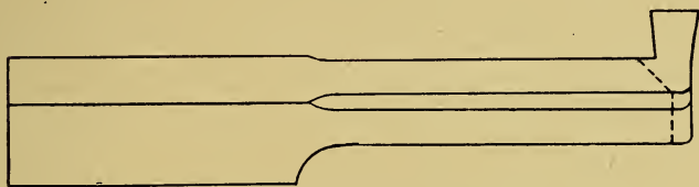
Fig. 44. The inside square thread tool.
