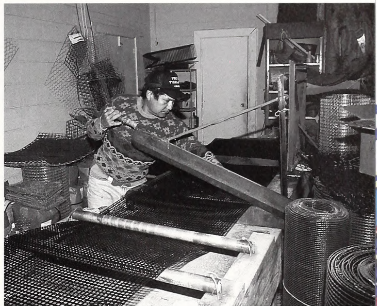
An employee cuts measured sections of wire mesh in preparation for the construction of new eel pots.
