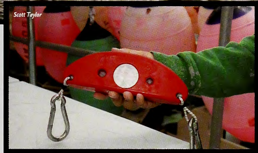
TOP: Each Save Wave has a microcomputer that produces sound either between 60-150 kHz or 5-90 kHz. BOTTOM: Lynne Williams uses a hydrophone to listen for echolocation behavior.
