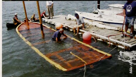
TOP TO BOTTOM: Construction drawings included a sail plan by Mike Alford. • By Spring 2003, construction was in advanced stages. • The builders put the finishing touches on the interior hull. • A large crew pushes off the dock to practice rowing trials in the Beaufort waterway. • Swamping tests are performed to see how well the Periauger floats when flooded with water.
