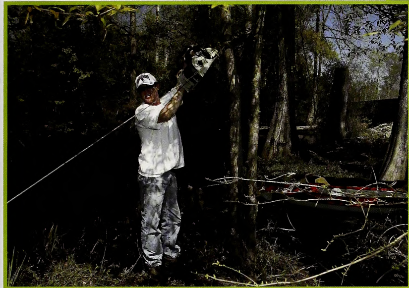
LEFT: Michael Banks demonstrates a small winch powered by a chainsaw motor, used to swing cut wood out of the channel. ABOVE: Connie Asero enjoys the sights along a section of the White Oak that was inaccessible before the project.
