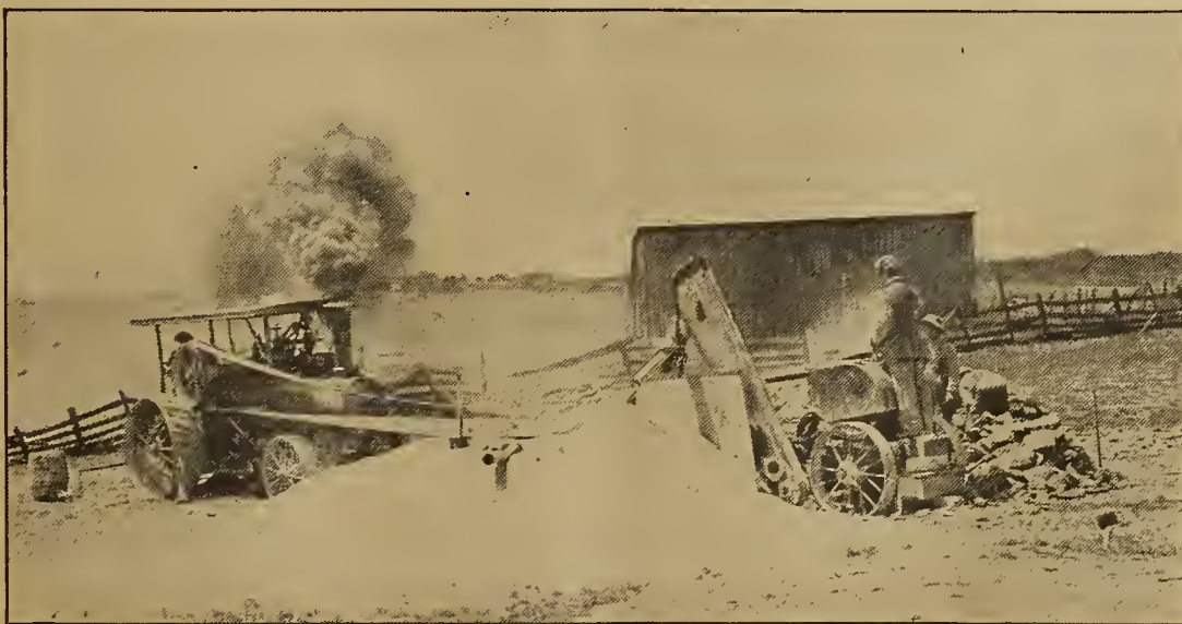
A limestone pulverizer costs from $450 to $1,000, and requires from eight horsepower up to run it. The average machine will pulverize about two tons of rock an hour
