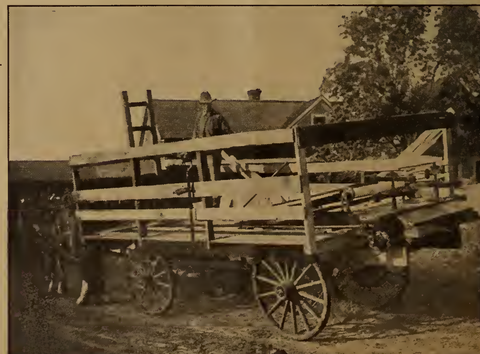
Here is a box rack equipped with a straw spreader. The straw is kicked out by the mechanism shown in the back
