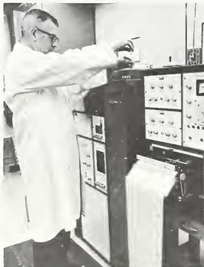
Gas chromatograph is used in basic research on control of insects that attack wood products (Wood Products Insect Laboratory, Gulf-port, Miss.)
