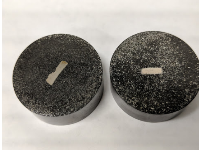
Figure 8. HIP Cu(micron)-Ni(micron) at 172 Mpa/1000°C
