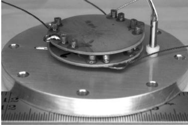
Figure 6.1. Mass-weighting of a two-disc driver.
