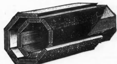
Two staves removed to show the lining between the inside and outside staves.
