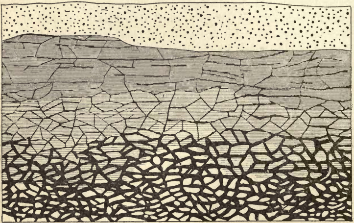
FIG. 8.—Section of the Hurst limonite bank, Wythe County, Virginia, illustrating the replacement of shattered limestone with limonite and the formation of geodes of ore. After E. R. Benton, Tenth Census , Vol. XV., p. 275.
