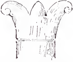
Etruscan Ionic capital, from a relief. Showing the central spike (erect sepal) and two curling sepals.
