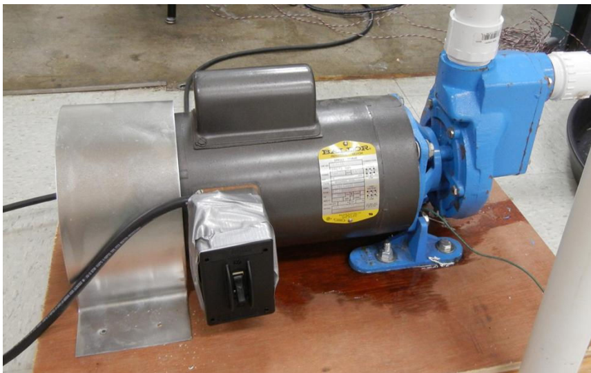
Figure 38. AC Motor Single Phase Pump
