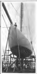
Bow View, emphasizing the Flat Keel and Flat Body
