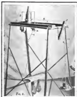
Diagram showing that the same Car with an increased Weight is propelled by a smaller Force
