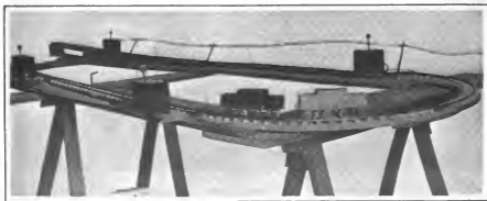
The boxes beside the miniature Track shown in the Photograph are the important Features of the System. In actual Service one of these Boxes will stop a Train by automatically setting the Brakes, and will also display a Sign indicating the Danger ahead—whether a Train on the Track, an open Switch, or a washed-out Bridge
