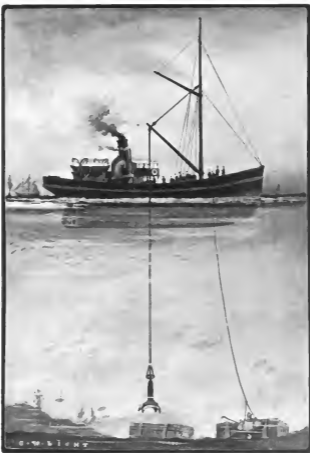
Using the new hydrographic invention of Signor Cavalliere Pino for exploring the bottom of the sea, the explorer is able to descend in the egg-shaped sink to great depths. The grappling device shown in the drawing is worked from the deck of the ship, from there, also, the life and treasures of the sea floor may be seen by means of a series of mirrors.
