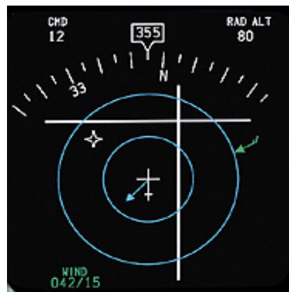
Figure 3. Rockwell-Collins Hover Display
