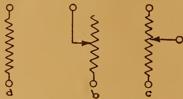
Figure 7—Resistances are shown in these drawings, one fixed, one variable, one of a special unit
