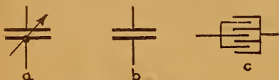
Figure 6—Three methods of showing condensers on diagrams, one variable and two fixed
