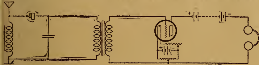
Figure 43—How an amplifier tube is used to increase the strength of signals from crystal detector
