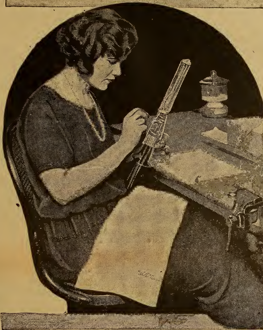
A girl's deft fingers formed the tongue with which S. S. Leviathan "speaks" at will by Radiotelegraph to either side of the ocean. Miss Marie Prepelik is seen assembling the "insides" of a 10,000-watt vacuum tube. Two of these furnish the power to the Leviathan's big Radiotelegraph transmitter which has power enough to span the Atlantic. Western Electric Photo
