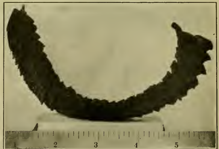
FIG. 4—CHIP TAKEN ON 36-INCH MIDVALE TIRE.
