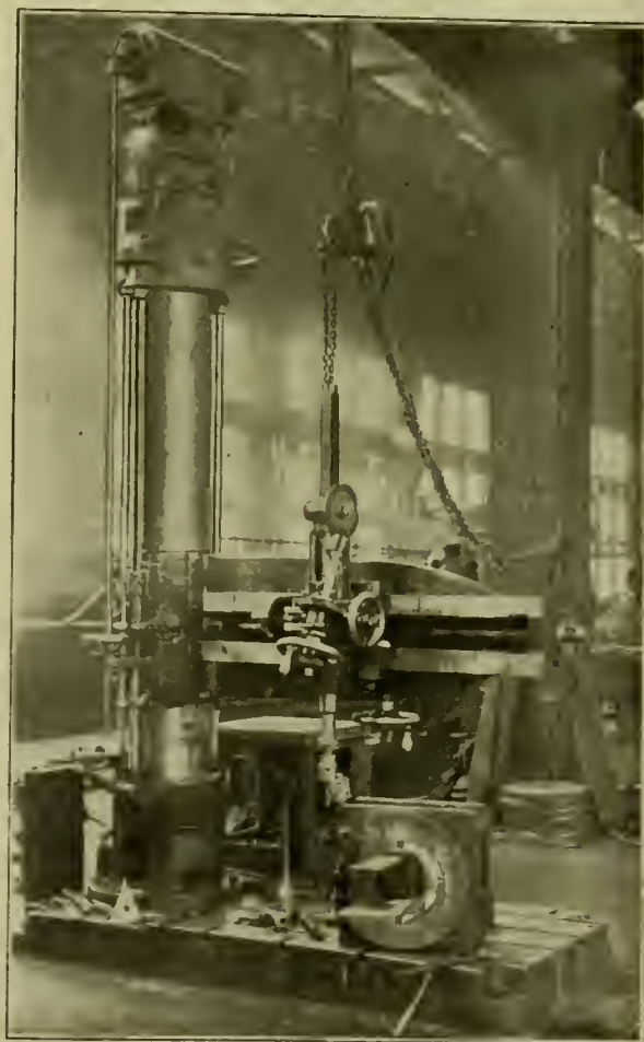
FIG. 5.—VERTICAL MOTOR APPLIED TO DRESES RADIAL DRILL.
