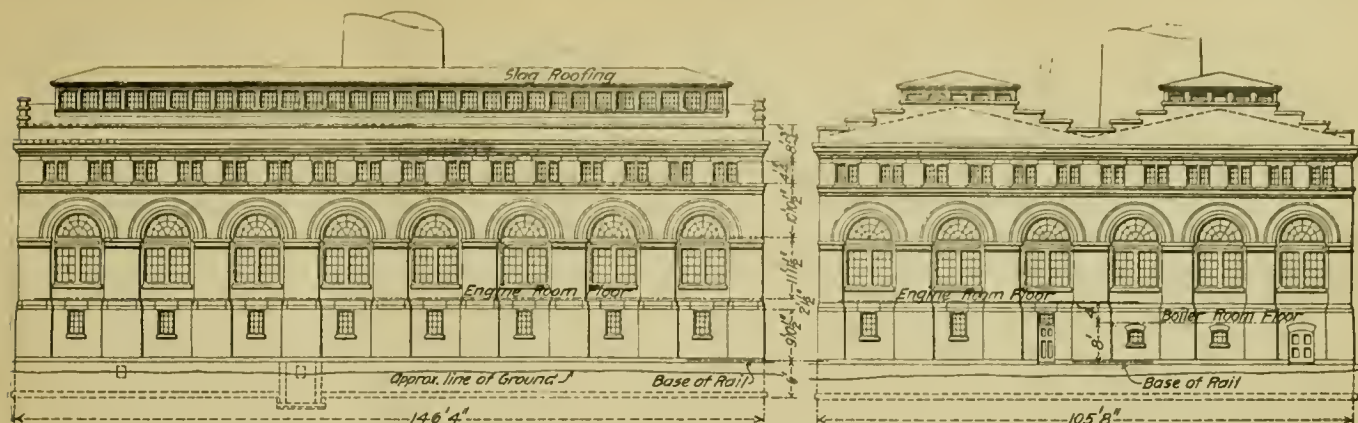
FRONT AND NORTH END ELEVATIONS OF THE POWER HOUSE, SHOWING CHARACTER OF CONSTRUCTION AND ARCHITECTURAL DETAIL. NEW TERMINAL YARD LIGHTING AND POWER PLANT.—WEST SHORE RAILROAD.
