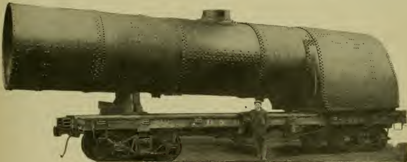
THE LARGEST LOCOMOTIVE BOILER IN THE WORLD. BUILT BY THE AMERICAN LOCOMOTIVE COMPANY. MALLET COMPOUND LOCOMOTIVE, BALTIMORE & OHIO RAILROAD.
