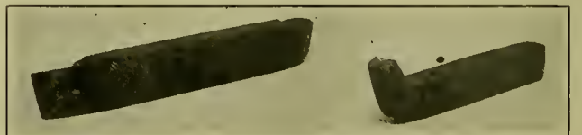
FIG. 4.—ROUGHING TOOLS. NEW ROUND NOSE, SUPPORTED CUTTING EDGE STYLE, AND OLD DIAMOND POINT, UNSUPPORTED STYLE.
