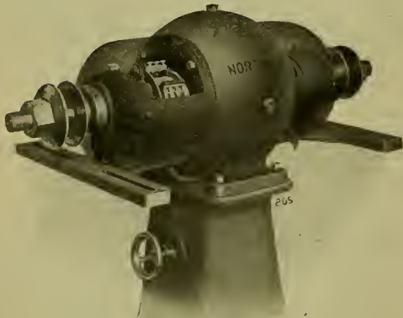
FIG. 18.—NORTHERN ELECTRIC EMERY GRINDER WITH TRANSPARENT COVER TO SHOW MOTOR.
