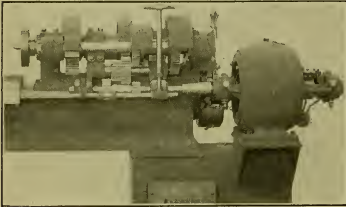
REAR VIEW OF LODGE & SHIPLEY LATHE SHOWING MOTOR APPLICATION.
