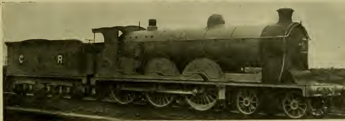
NEW SIX COUPLED PASSENGER LOCOMOTIVE.—CALEDONIAN RAILWAY.
