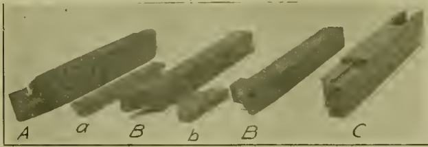
FIG. 11.—TOOL HOLDER FOR USE ON WHEEL LATHES AND SOLID TOOLS DISPLACED BY SAME.
