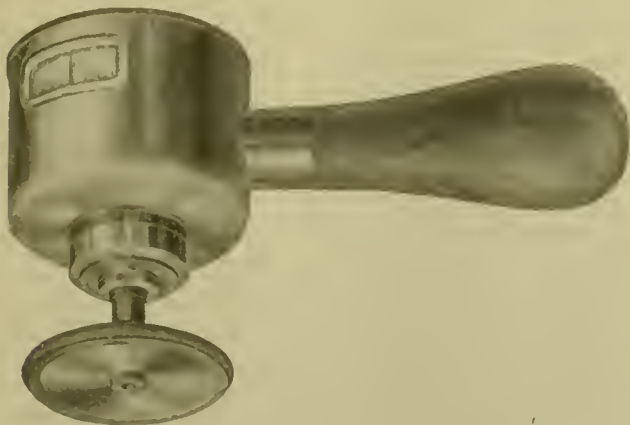
VIEW OF THE CUT-METER, AS USED FOR MEASURING CUTTING SPEEDS ON MACHINE TOOLS.
