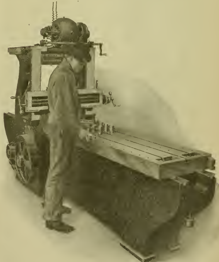
METHOD OF USING THE CUT-METER TO INDICATE THE TABLE SPEED OF A PLANER.—GIVES EXACT CUTTING SPEED INSTANTLY WITHOUT CALCULATIONS.
