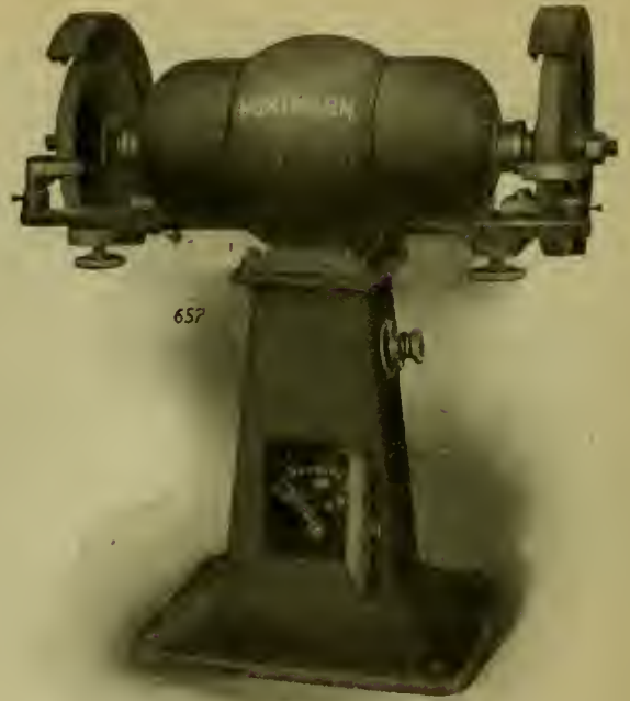
FIG. 17.—MOTOR-DRIVEN EMERY GRINDER—NORTHERN ELECTRIC MANUFACTURING COMPANY.
