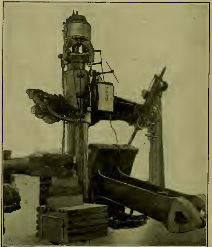
FIG. 2.—SPECIAL NILES PORTABLE FLOOR PLATE DRILL, WITH DIRECT VERTICAL-MOTOR DRIVE; AT THE WORKS OF THE BULLOCK ELECTRIC MFG. COMPANY.
