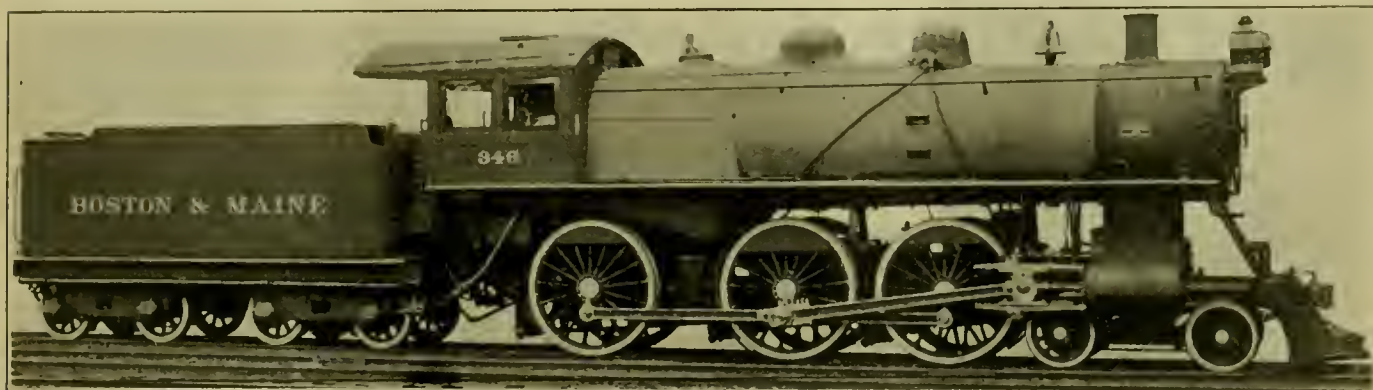
SIX-COUPLED PASSENGER LOCOMOTIVE.—BOSTON & MAINE RAILROAD.—4-6-0 TYPE.—WIDE FIREBOX OVER 72-IN. DRIVING WHEELS.
