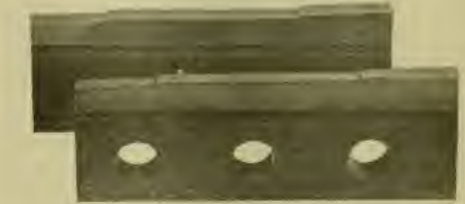
FIG. 9.—FORMING TOOLS USED ON WRIST PIN.
