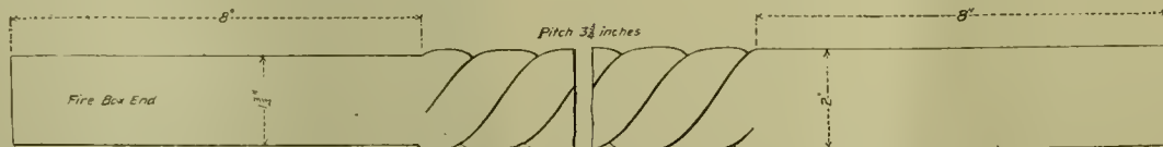
SPIRALLY CORRUGATED BOILER TUBE.
