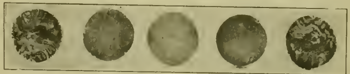
ETCHED SECTIONS OF STAY-BOLTS.
