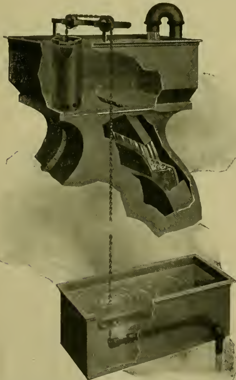
DIAGRAMMATIC VIEW OF THE FLOAT MECHANISM FOR VARYING THE HEIGHT OF THE ORIFICE IN THE TANK OUTLET PIPE, AS USED TO CONTROL THE RATE OF FLOW OF THE CHEMICAL SOLUTIONS.
