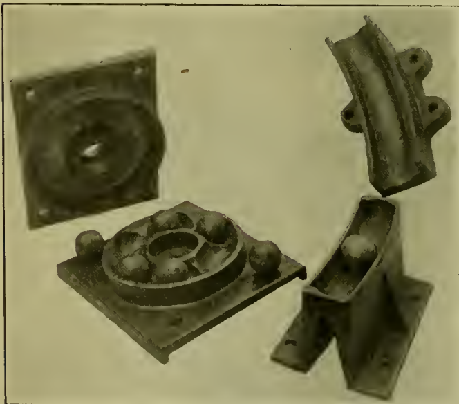
HARTMAN BALL BEARING CENTER PLATES AND SIDE BEARINGS.
