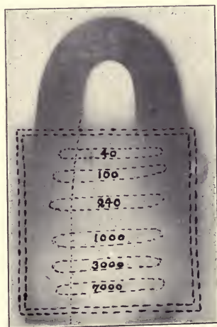
FIG. 8.—Radiograph showing Degrees of Penetration of a thick sheet of Lead and a Steel Magnet by Tubes of Radium of Different Radioactivities
