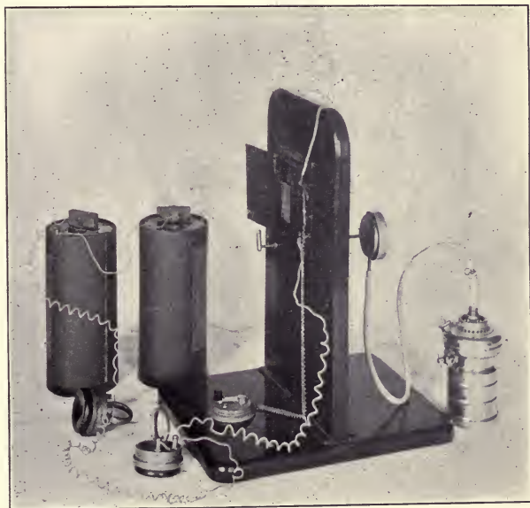
FIG. 20.—Manometric Acetylene Flame Transmitter with Selenium Cell, etc.—(a battery of about 24 volts employed).
