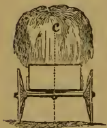
Centre of gravity on level and inclined roads.
