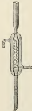
THE KOBE CONDENSER. The connection is made by means of an annular groove in the key
