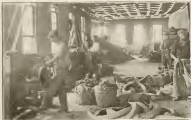
(The Loewenthal Co.) PULLING FABRIC FROM TIRE CARCASSES. THE TREAD STOCK WINDS ON THE DRYUM WHILE THE PULLED FABRIC WINDS ON THE SPINDLE, EACH IN OPPOSITE DIRECTIONS. THE PRODUCTS MAY BE NOTED ON THE FLOOR AND IN THE BASKETS.
