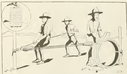
UNITED STATES ARMY METHOD OF STRIPPING SOLID TRUCK TIRES. HEAT PROCESS SHOWN IN INSERT.
