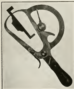
THE 3-INCH INDICATING CALIPER.
