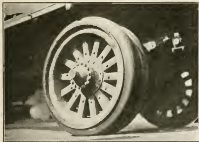
SOLID TIRES ARE INDISPENSABLE IF DELIVERY OF THE LOAD MUST REACH ITS DESTINATION WITHOUT FAIL AT TIME PROMISED; IF REGULAR DELIVERY IS MORE IMPORTANT THAN EITHER SPEED OR COST OF DELIVERY, OR IF THE CAR CARRIES OVERLOADS BEYOND THE RATED CAPACITY OF THE TIRES.
