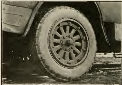
PNEUMATIC TIRES ARE IMPERATIVE UNDER SOME COMBINATION OF THE FOLLOWING FACTORS: TRACTION ON ANY KIND OF ROAD SURFACE, OR OFF THE ROAD, WITH COST SUBORDINATED; SPEED WITH COST SUBORDINATED, OR WHEN PROTECTION OF MERCHANDISE FROM ROAD SHOCK IS ESSENTIAL.
