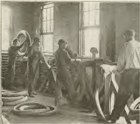
(The Lowenthal Co.) STARTING FABRIC PLYS. THE SUCCESSIVE STEPS MAY BE NOTED FROM LEFT TO RIGHT IN THE PICTURE, COMPRISING REVERSING THE TIRE, CUTTING, AND STARTING THE PLYS TO BE PULLED.
