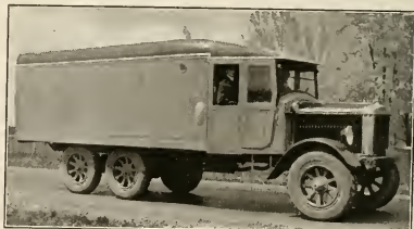
INSTEAD OF TWO GIANT PNEUMATIC TIRES, EACH WEIGHING 398 POUNDS, THE TANDER AXLE CONSTRUCTION PERMITS THE USE OF FOUR 40 BY 8 PNEUMATIC TIRES, EACH WEIGHING ONLY 119 1/2 POUNDS.
