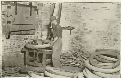
(The Lowenthal Co.) CUTTING BEADS FROM TIRE CASINGS. A PARTLY SEVERED BEAD IS SEEN CUTTING UPWARD FROM THE CIRCULAR KNIFE, AND IN THE BACKGROUND IS A PILE OF CUT BEADS.
