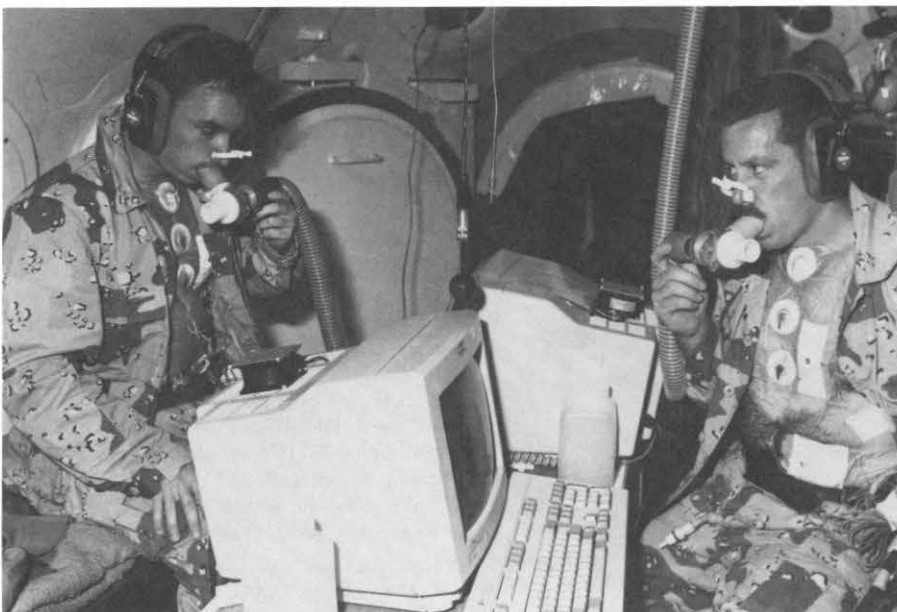
Divers during "dry phase." Note computer terminals for testing with the PAB. Divers are breathing into the spirometry circuit to measure respiratory volumes and oxygen consumption.
